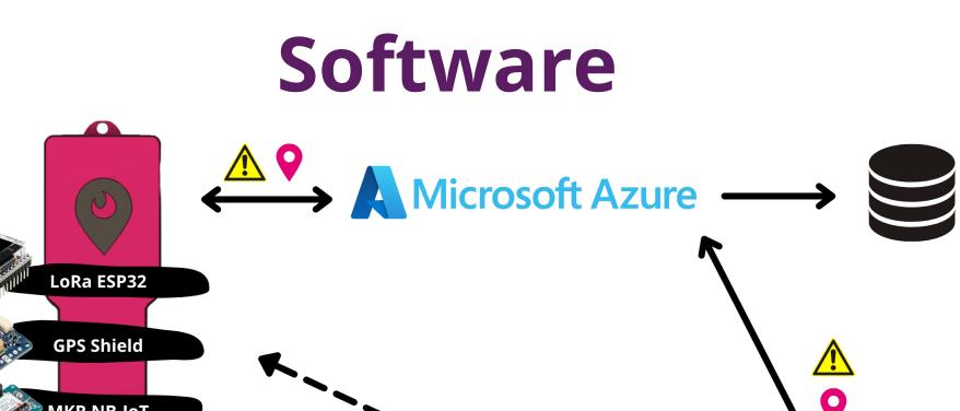
Cellular data is shared between devices and stored in table storage using the Azure IoT Hub. LoRa data is stored locally on the user's mobile app.
